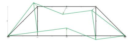
Fig. 5.33 Possible infinitesimal motions in a frame can be discovered with the "twofold" Gauss
