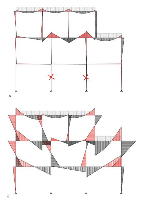
Fig. 5.32 One-click reanalysis (without modification of the stiffness matrix), **a** the crossed-out elements, **b** moment distribution without the two columns
